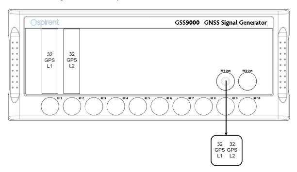
Figure 4 Example of a single output, 2-bank system GPS L1 L2
