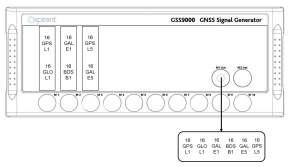
Figure 5 Example of a single output, 3-bank system
