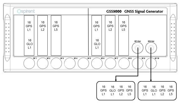
Figure 6 Example of a dual-RF Output, 6-bank system
